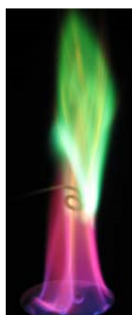
Copper(II) Chloride colors a cool ethanol flame a vivid green.
