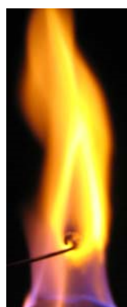
Sodium Chloride imparts a bright, strong, yellow color to an ethanol flame.
