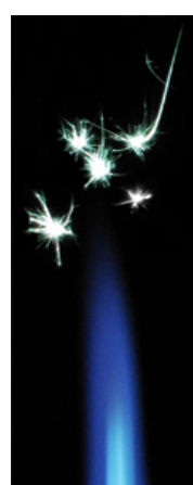
Small Magnesium metal turnings burn above a butane flame (Left) and ethanol flame (Right).
