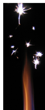
Small Magnesium metal turnings burn above a butane flame (Left) and ethanol flame (Right).
