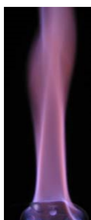
An ethanol flame is colored a light purple / lilac by Potassium Chloride.
