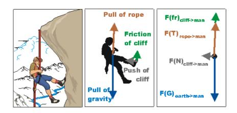
2. Free Body Diagram (FBD) - Only the object being analyzed is drawn. Uses arrows to show all the forces acting on the object.
