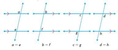
When a transversal intersects a pair of lines creating equal corresponding angles, the pair of lines is parallel.
