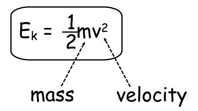
This equation means that things that are heavier or going faster can carry a higher kinetic energy.
